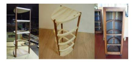
The box-shaped lute was drawn to the PC, and its construction is quite elaborate, I have made of birch cut ribs with numerical control milling machine then assembled and glued to 3 pillars of mahogany wood. The structure thus obtained was "wrapped" before by a panel of lead 1 mm thick, then with 5 bendable sheets of wood with a thickness of 5 mm each glued with vynil glue.
