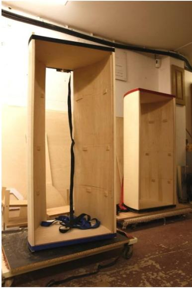
Side panels Glued to base and top panels. At this stage, the veneer had already been applied to the side panels in the vacuum former as that was the best way to achieve a bubble free veneer!
