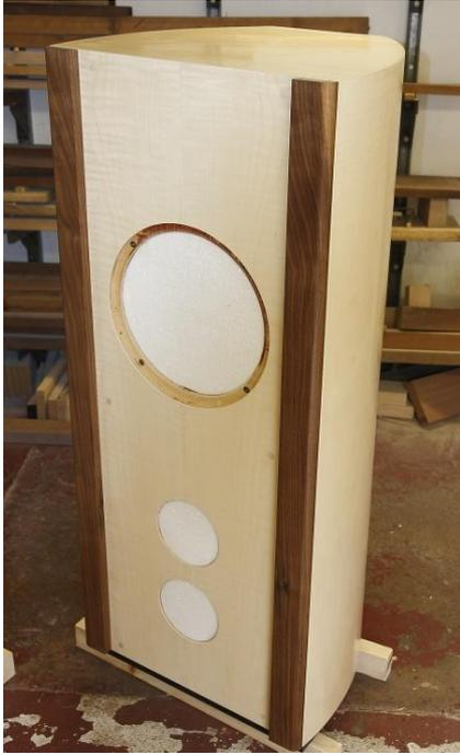
Baffle glued into position and baffle edge strips (oiled American Black Walnut) added. The grille will fit neatly in between the edge strips which have rounded edges on the corners of the baffle to improve baffle performance. The top of the cabs has now been veneered and a 50mm curved plinth added to the base.
