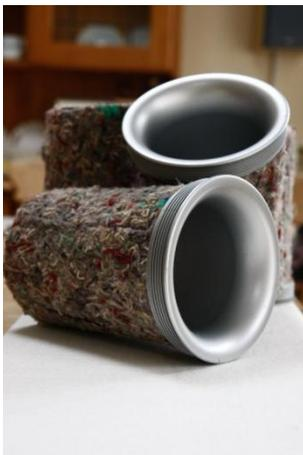
Ports before spraying black and extending with some uPVC pipe couplers (flared at the ends using a heat gun and former). I glued some wool felt to these again in my obsessive target of controlling internal reflections, possibly overkill though.
